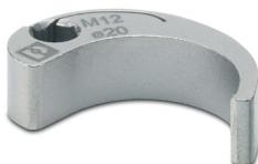
Nut for assembling M12 connectors for assembly with a knurl diameter of 20 mm, for 4 mm hexagonal drive
